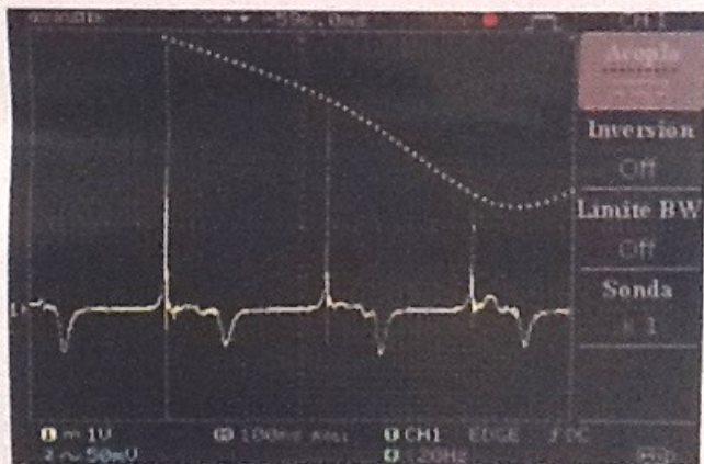
Figure 4. Response signal of the inductive sensor.
