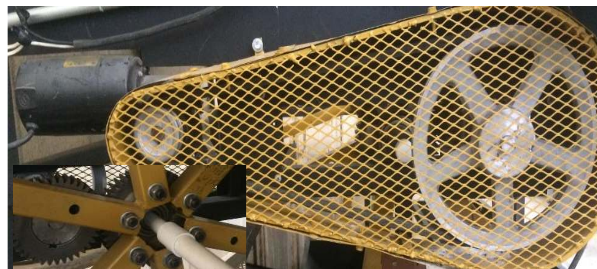
Figure 2. Motor, pulleys and gears of the vertical greenhouse
