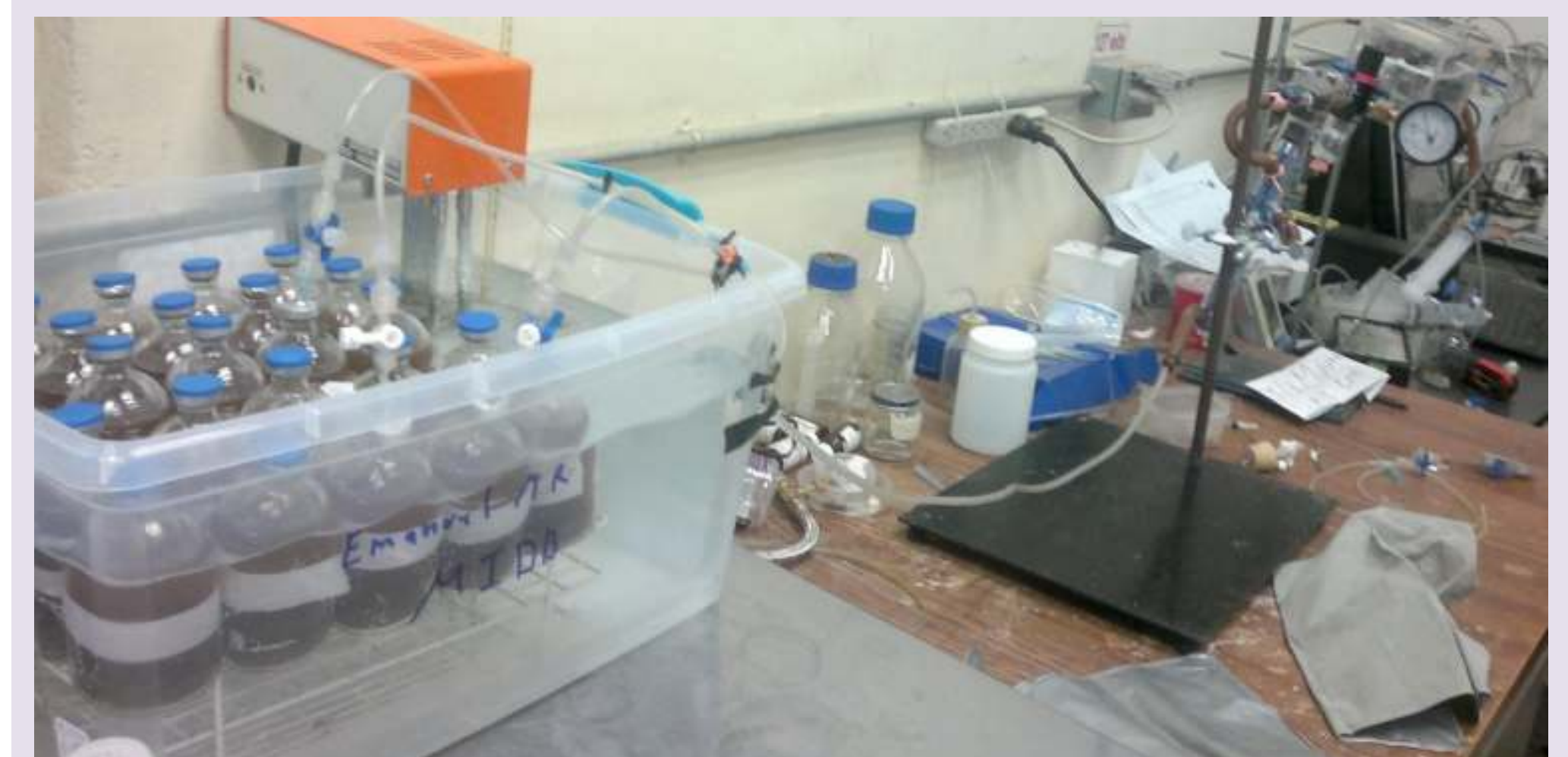
Figure 6. Online monitoring of horse manure anaerobic digestion
