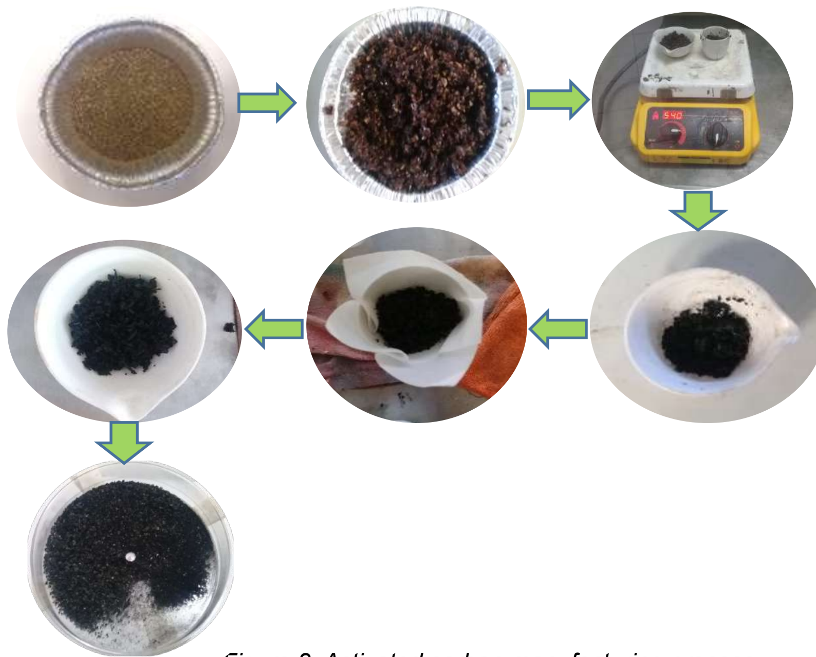
Figure 8. Activated carbon manufacturing process.
