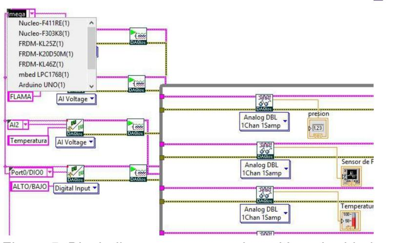
Figure 8. Graphical interface for monitoring and data acquisition in LabVIEW.
