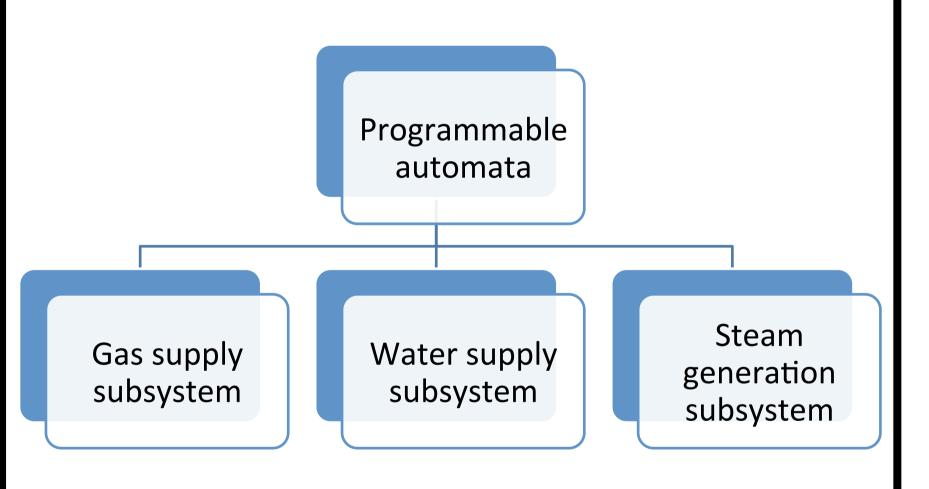
Figure 4. Block diagram of the integral automatic control system of steam generators [3].
