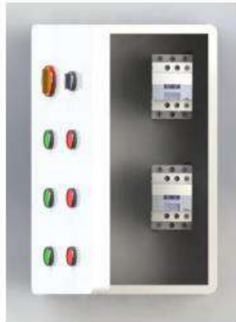
Figura 3.5 Tablero de control real
