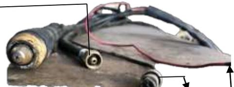
Figura 7: Antorcha. Cable inhabilitado
