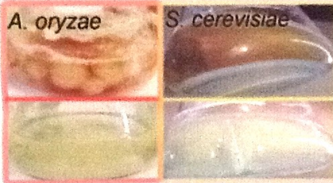
Figure 2. Growth in flask at pH=7 and sterilized on top and growth at pH=4 and pasteurized on bottom.
