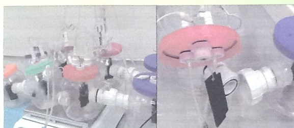
Figure 3. Left prototypes of MFC developed. Right: components of the MFC
