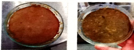
Figure 5. Plastic obtained using banana peel. On the left using yellow shells unpigmented and right with more mature shells.
